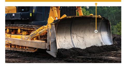
Three intelligent blade speed modes – slow, neutral and fast – perfectly calibrate to match and adjust the blade speed to your application, increasing your accuracy and precision.
